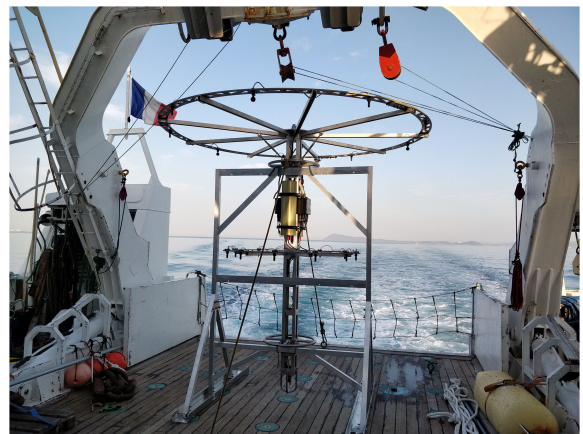
Fig. 7. Final acoustic array obtained. Height: 2.7 \text{ m} ; largest width: 2.9 \text{ m} . It is composed of 17 HTI-96-MIN and 4 Neptune D/60 hydrophones. (Credits: OSEAN SAS).
