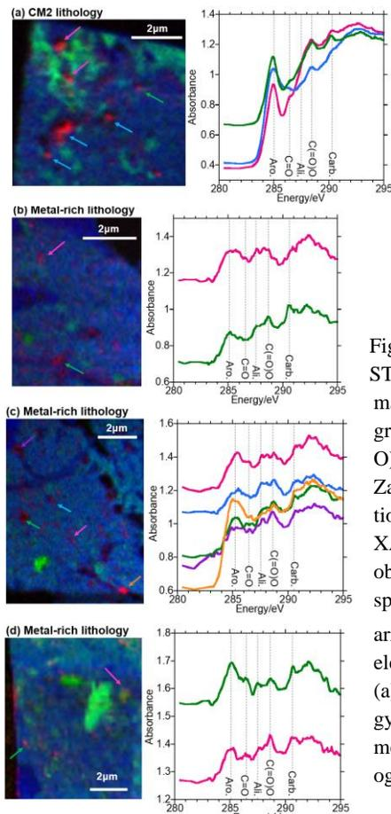
Fig. 2: (Left) STXM elemental maps (red: C, green: Fe, blue: O) of the Aguas Zarcas FIB sections. (Right) XANES spectra obtained from the spots indicated by arrows in the elemental maps. (a) CM2 lithology, and (b-d) metal-rich lithology.
