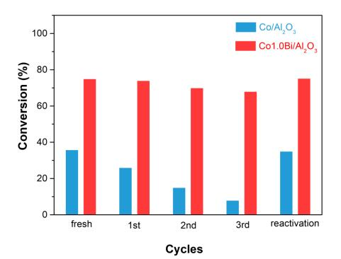
**Figure 4** Catalytic reusability and stability for liquid phase amination of 1-octanol over activated Co/Al<sub>2</sub>O<sub>3</sub> and Co1.0Bi/Al<sub>2</sub>O<sub>3</sub> catalysts (1-octanol, 0.84 g; molar ratio of 1-octanol/NH<sub>3</sub>/H<sub>2</sub> = 1/4.5/0.85; P<sub>H2</sub> = 3 bar; catalyst amount, 100 mg; reaction temperature, 180 °C; time, 5 h; no solvent used; reactivation condition: 400 °C calcination under air followed by H<sub>2</sub> activation at 450 °C).
