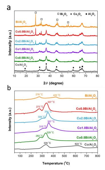
Figure 5 XRD patterns (a) and  $H_2$ -TPR profiles (b) of oxidized Co/Al<sub>2</sub>O<sub>3</sub>, Bi/Al<sub>2</sub>O<sub>3</sub> and bimetallic Co*x*Bi/Al<sub>2</sub>O<sub>3</sub> catalysts.
