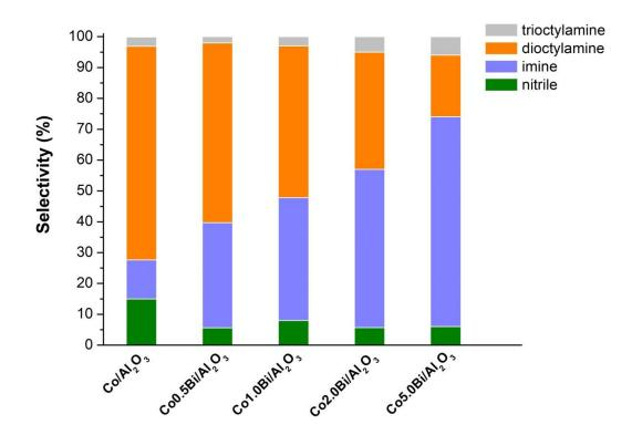
**Figure 8** Model reaction of 1-octylamine transformation over activated Co/Al<sub>2</sub>O<sub>3</sub> and bimetallic CoxBi/Al<sub>2</sub>O<sub>3</sub> catalysts at a conversion of < 10% (1-octylamine, 1 mL; catalyst amount, 20 mg; molar ratio of 1-octanol/NH<sub>3</sub>/H<sub>2</sub> = 1/4.5/0.85;  $P_{H_2}$  = 3 bar; reaction temperature, 180 °C; time, 0-4 h; no solvent used).
