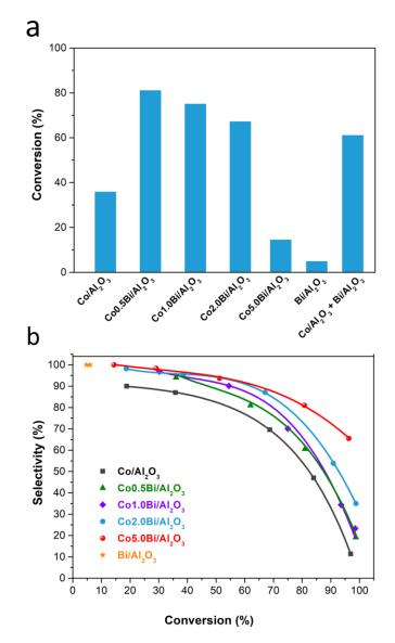
**Figure 3** Catalytic conversion modification by Bi promotion (a) and selectivity-conversion curves (b) for liquid phase amination of 1-octanol over activated Co/Al<sub>2</sub>O<sub>3</sub> and bimetallic CoxBi/Al<sub>2</sub>O<sub>3</sub> catalysts (1-octanol, 0.84 g; molar ratio of 1-octanol/NH<sub>3</sub>/H<sub>2</sub> = 1/4.5/0.85; P<sub>H2</sub> = 3 bar; catalyst amount, 100 mg; reaction temperature, 180 °C; time, 0-48 h; no solvent used).
