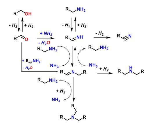
Figure 2 Reaction paths in amination of alcohols over supported metal catalyst
