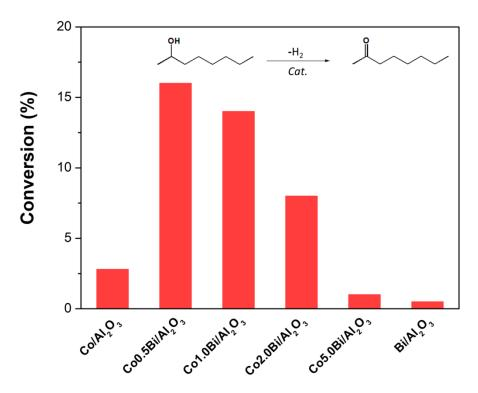
**Figure 7** Comparison of catalytic conversion for liquid phase dehydrogenation of 2-octanol over activated  $Co/Al_2O_3$ ,  $Bi/Al_2O_3$  and bimetallic  $CoxBi/Al_2O_3$  catalysts (2-octanol, 50 mg; toluene, 1 g; catalyst amount, 50 mg; reaction temperature, 140 °C; time, 15 h).
