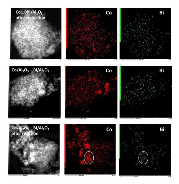
**Figure 6** HAADF-STEM images and EDX mapping of Co and Bi of reduced Co1.0Bi/Al<sub>2</sub>O<sub>3</sub> catalyst and mechanical mixture Co/Al<sub>2</sub>O<sub>3</sub>+Bi/Al<sub>2</sub>O<sub>3</sub> before and after reaction of amination
