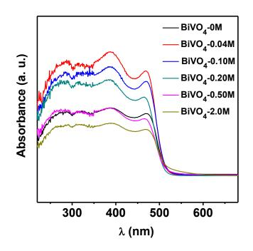
Figure 4. UV-Vis spectra of BiVO<sub>4</sub> samples synthesized with different concentration of NaCl.
