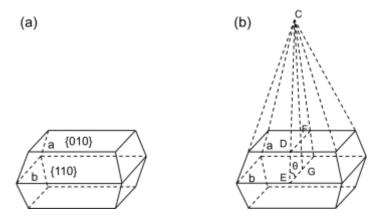
**Figure 3.** Crystal model of monoclinic BiVO<sub>4</sub> crystals with truncated tetragonal bipyramidal shape.
