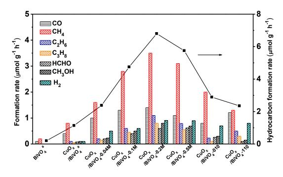
**Figure 10.** Effect of the fraction of  $\{010\}$  facets on the photocatalytic performance of  $CuO_x/BiVO_4$  catalyst for reduction  $CO_2$  with  $H_2O$ . <sup>a</sup>  $BiVO_4$  with an irregular morphology (NaCl concentration: 0M).
