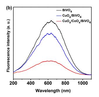
**Figure 5.** (a) Photoluminescence spectra of BiVO<sub>4</sub> samples synthesized with different concentration of NaCl. (b) Photoluminescence spectra of BiVO<sub>4</sub>-0.20M crystal with selective photo-deposited the metal oxides.
