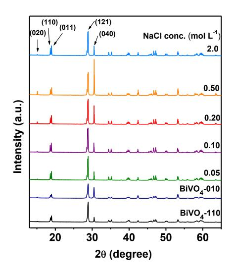
**Figure 1.** *XRD patterns of the monoclinic BiVO*<sup>4</sup> *samples with different concentration of NaCl and BiVO*<sup>4</sup> *with predominately exposed {010} and {110} facets*
