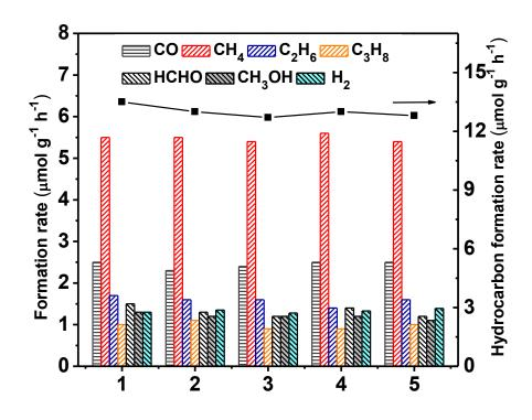
**Figure 12.** Repeated uses of the 5 wt%  $CuO_x/5$  wt%  $CoO_x/BiVO_4$ -0.20M catalyst for photocatalytic reduction of  $CO_2$  with  $H_2O$ .
