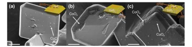
**Figure 8**. SEM images of BiVO<sub>4</sub>-0.20M sample with selective photo-deposited metal oxides: (a) CuO<sub>x</sub>/BiVO<sub>4</sub>, (b) CoO<sub>x</sub>/BiVO<sub>4</sub>, (c) CuO<sub>x</sub>/CoO<sub>x</sub>/BiVO<sub>4</sub>.
