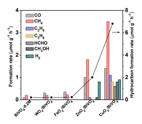
**Figure 9.** *Effect of metal oxides on the performance of BiVO*<sub>4</sub>*-0.20M for photocatalytic reduction CO*<sub>2</sub> *with H*<sub>2</sub>*O.*
