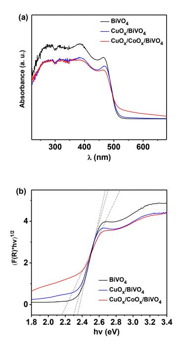
**Figure 6** a. UV-Vis spectra of  $CuO_x/CoO_x$  /BiVO<sub>4</sub>-0.20M sample b.  $[F(R\infty)hv]^{1/2}$  versus hv
