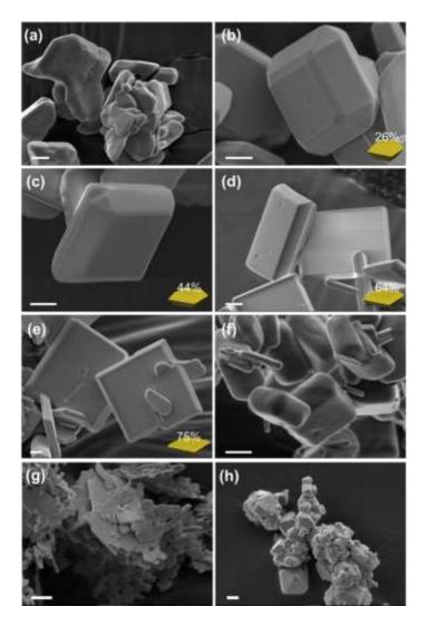
**Figure 2.** SEM images of BiVO<sub>4</sub> samples synthesized with different concentration of NaCl. NaCl concentration: (a) 0 M, (b) 0.04 M, (c) 0.10 M, (d) 0.20 M, (e) 0.50 M, (f) 2.0 M, (g) BiVO4-010, (h) BiVO4-110. Scale bar: 1.0 µm.
