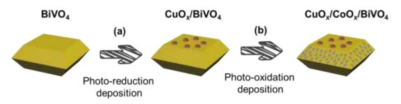
**Figure 7**. Schematic of the synthesis of CuO<sub>x</sub>/CoO<sub>x</sub>/BiVO<sub>4</sub> catalyst.
