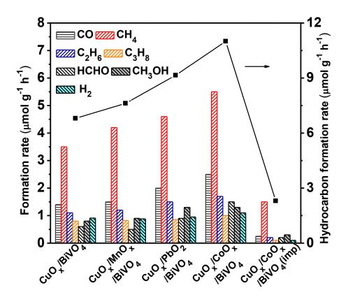
**Figure 11.** Effect of cocatalyst on the performance of  $CuO_x/BiVO_4$ -0.20M for photocatalytic reduction  $CO_2$  with  $H_2O$ .
