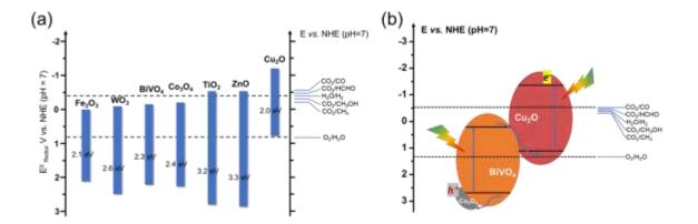
**Figure 13.** (a) Comparison of the band structures of various semiconductor with respect to the redox potentials of reduction of  $CO_2$ , (b) Schematic of the Z-scheme of  $CuO_x/CoO_x/BiVO_4$ -0.20M catalyst.
