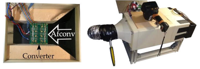
Figure 4. Left: Picture of a MCC under test inside the wind tunnel. Right: Fully instrumented characterization bench [PCIM].
