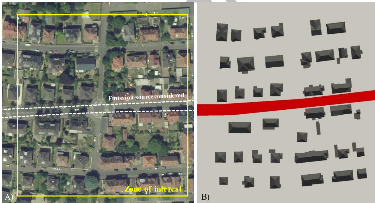
159 160 Fig. 4. Illustration of (A) the area of Strasbourg modeled with the road considered for the traffic-related emissions (white 161 dashed lines), and (B) the corresponding area built in 3D for the numerical simulations with the emission source (red).
