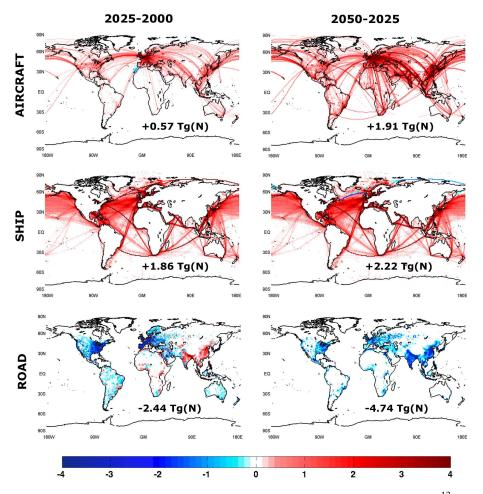
**Fig. 1.** Spatial distribution of the absolute difference in NO<sub>x</sub> emission flux for the SRES A1B scenario (units:  $10^{13}$  molecules NO<sub>2</sub> m<sup>-2</sup> s<sup>-1</sup> for AIRCRAFT and SHIP;  $10^{14}$  molecules NO<sub>2</sub> m<sup>-2</sup> s<sup>-1</sup> for ROAD).
