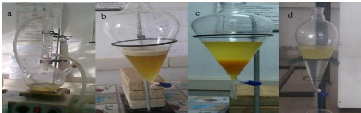
**Figure 1. (a) First stage esterification process. (b) Separation of gum and sticky materials after first stage (c) Separation of glycerol after second stage transesterification (d) Water washed methyl ester after second stage of transesterification**
