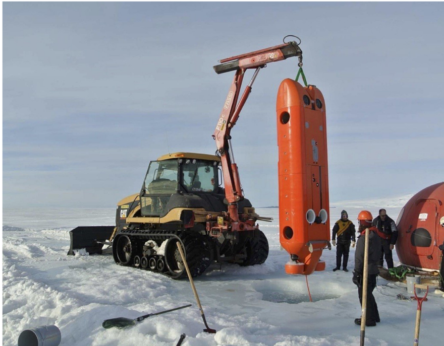
FIGURE 4 | Stone Aerospace's ARTEMIS vehicle being launched into the Antarctic ocean through a drilled hole.
