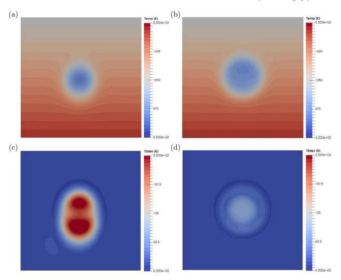
**Figure 8.** Upper panel: cross-sectional view in the *yz*-plane of the mean temperature field recovered from (a) isotropic inversion, and (b) anisotropic inversion. Lower panel: standard deviations around the mean temperature fields from (c) isotropic inversion and (d) anisotropic inversion. These cross-sections are taken at the centre of the *x*-axis.
