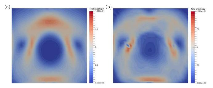
Figure 11. Cross-sectional view in the yz-plane of the percentage of total anisotropy (i.e. norm of  $S_{ij}$ ) inferred from (a) true model and (b) mean model. The absence of anisotropy at the centre corresponds to a region of minimal deformation for the cold and highly viscous anomaly. The cross-sections are taken at the centre of the x-axis.
