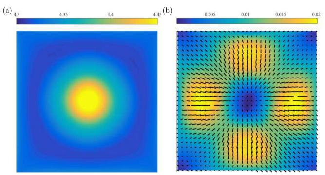
Figure 4. Phase velocity maps resulting from one sinking anomaly at 100 s period. (a) Rayleigh wave phase velocity  $(km s^{-1})$ . (b) Azimuthal anisotropy in Rayleigh waves  $(km s^{-1})$ . The solid black lines correspond to the direction of the fast propagation axis. Surface wave maps always lie along the *xy*-lateral plane.
