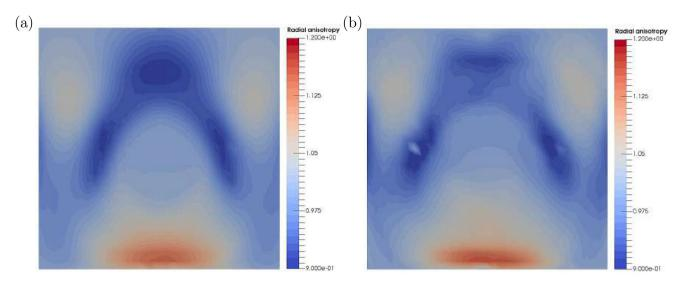
**Figure 10.** Cross-sectional view in the *yz*-plane of the radial anisotropy  $\xi$  inferred from (a) true model and (b) mean model. Radial anisotropy is often used as a proxy to infer flow orientation. A  $\xi > 1$  (positive radial anisotropy) is often interpreted as horizontal flow. A  $\xi < 1$  (negative radial anisotropy) on the other hand, pertains to vertical flow. A  $\xi = 1$  indicates the absence of radial anisotropy. The cross-sections are taken at the centre of the *x*-axis.
