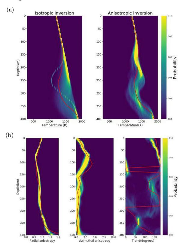
**Figure 14.** Upper panel: comparison between isotropic and anisotropic inversion. Probability density plots of temperature with depth. The profiles are taken nearly through the centre of the sphere. Lower panel: anisotropic inversion: probability density plots of radial anisotropy, peak-to-peak azimuthal anisotropy and its fast axis with depth. All profiles correspond to the temperature profile above. The solid red lines indicate the true structures.
