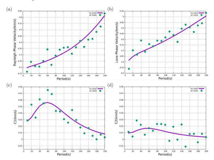
Figure 5. Synthetic surface wave dispersion curves from 10 to 200 s at a given location: (a) Rayleigh wave phase velocity, (b) Love wave phase velocity, (c) Rayleigh anisotropy  $c_1$  and (d) Rayleigh anisotropy  $c_2$ . Scatter plot: observed dispersion curve with added noise. Line plot: observed dispersion curve without noise.
