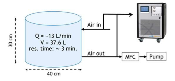
Fig.2: Photo of the analytical set-up, on the left on the table the Teflon analytical chamber containing a film and on the right the PTR-ToF-MS.
