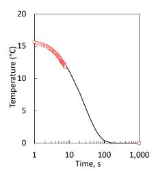
**Figure 3.** Temperature versus time after rapid loading at 1.s<sup>-1</sup> and rupture of the rubber specimen. The fitting law is an exponential function whose characteristic time is used to define the diffusion time on the rubber specimen surface.
