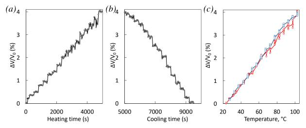
**Figure 1.** Volumetric dilatation (in %) due to external heating measured by DIC performed on front and side surfaces of the rubber specimen during heating/cooling at 10K.min<sup>-1</sup>. Volumetric dilatation has been measured during heating (a) and cooling (b) as a function of the time. The comparative evolution of volumetric strain during cooling/heating is presented in figure (c).
