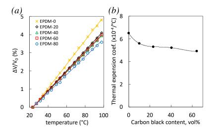
**Figure 4.** (a) Volumetric deformation due to thermal dilatation measured by DIC performed on surface of the rubber specimen, (b) Thermal expansion coefficients deduced from figure 4a for a series of EPDM with various carbon black contents from 0 to 80 phr (per hundred rubber).
