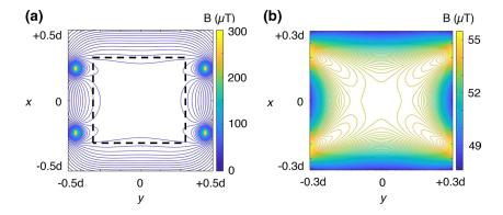
**Figure 3.** Simulation of the magnitude of compensation field in the z = 0 plane of a two-axis square Helmholtz coil system. (a) Contour plot of the field intensity inside the *z* coils with length *d*. The four areas of high field strength are at the intersections of the *x* coils with the central plane (*x* coils are inside the *z* coils). Dashed area is plotted in (b). (b) Contour plot of the field intensity inside the central area of the system where the field is most uniform.
