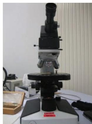
**Microscope polarisant Leica**
