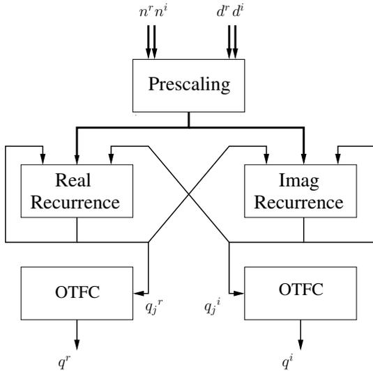
Fig. 1. Block Diagram of Complex Division using Recurrence.
