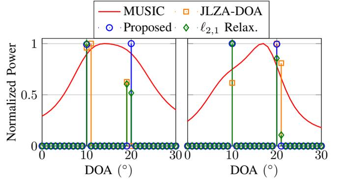
Fig. 3: Normalized power spectra for two realizations of noise with  $L = 40$  and SNR=10 dB (zoom between  $0^\circ$  and  $30^\circ$ ). The true DOAs are  $\bar{\theta}_1 = 10^\circ$  and  $\bar{\theta}_2 = 20^\circ$ .
