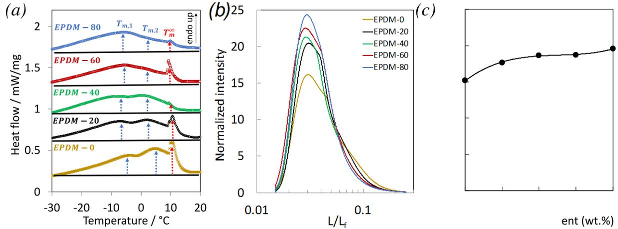
**Figure 6.** (a) DSC thermoporosimetry heating for undeformed EPDM-0, EPDM-20, EPDM-40, EPDM-60 and EPDM-80. Blue dotted arrows indicate the trapped solvent melting peaks ( $T_{m,1}$  and  $T_{m,2}$ ) and red dotted arrows indicate the free solvent melting peak, (b) Normalized intensity versus normalized pore size giving the pore size distribution (see section 2.4), (c) Network chain densities of filled EPDM calculated from equation (11).
