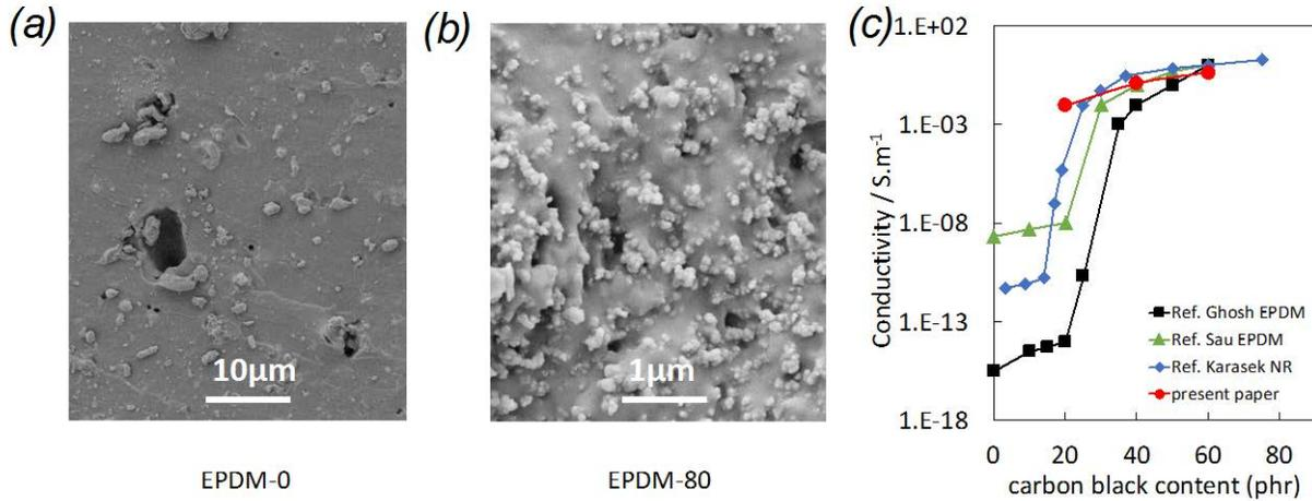
**Figure 4.** (a),(b) SEM images of cross-section of fractured EPDM-0 and EPDM-80 sample respectively, (c) Electrical conductivity versus carbon black content. The abrupt change in the conductivity is noted as the electrical percolation threshold, as shown in Refs. [27],[28],[29].
