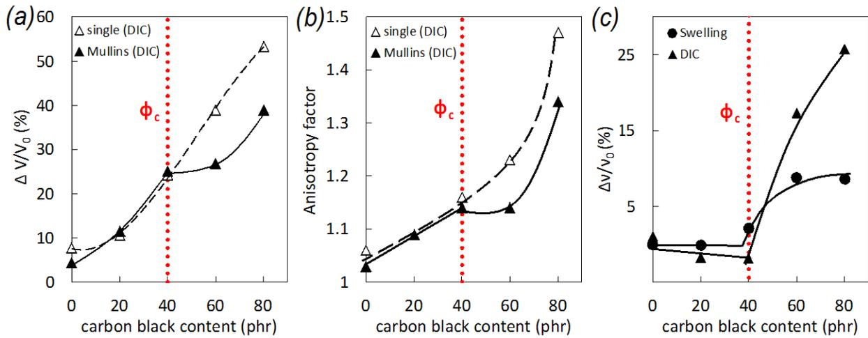
**Figure 10.** (a) DIC volumetric strain versus filler content for single and Mullins type tests measured at maximum strain, (b) corresponding anisotropy factor, (c) network chains density measured from swelling (Q) and DIC (V) for EPDM-0, EPDM-40 and EPDM-80 in undeformed state and stretched up to maximum extension.
