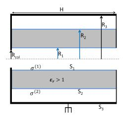
FIG. 1: Cut of the capillary along the xOz plane containing the symmetry axis. Black fat lines stand for grounded surfaces, namely the  $S_3$  interface, the entrance and the outlet of the capillary. Grey rectangles represent the dielectric bulk. Blue lines stand for vacuum-insulator interfaces of the inner  $(S_1)$  and outer  $(S_2)$  capillary surface, carrying the surface charge densities  $\sigma^{(1,2)}$ .
