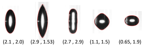
FIG. 2: Fit parameters (a/b, n) found for various observed shapes using the superellipsoid equation (34). Red contours show the corresponding superellipsoid shape.
