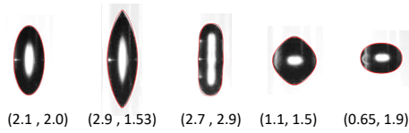
FIG. 2: Fit parameters (a/b, n) found for various observed shapes using the superellipsoid equation (34). Red contours show the corresponding superellipsoid shape.
