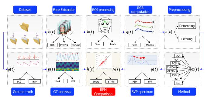
FIGURE 1: Overall pyVHR framework schema.
