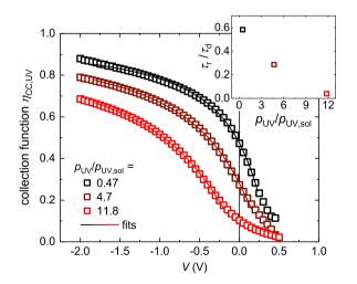
**Figure 5.** Voltage dependence of the carrier collection efficiency of a ZnO/eclipse-NiO solar cell under monochromatic UV excitation for different illumination intensities, and fits according to Equation (6).
