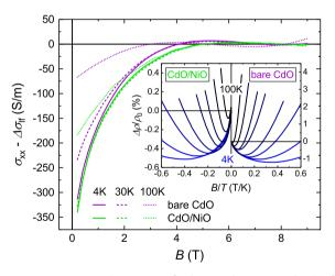
**Figure 11.** Magnetoconductivity  $\sigma_{xx}$  for bare and NiO-coated CdO for selected temperatures, after correction for positive Lorentz-force contribution. Inset: plot of MR versus *B*/*T* of both samples for all temperatures investigated.
