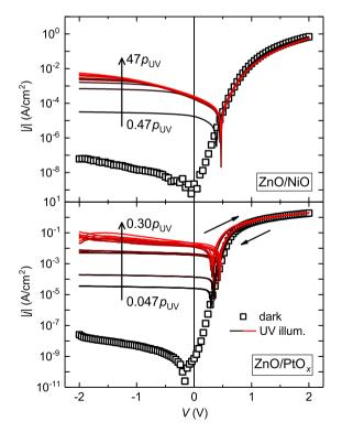
**Figure 4.** Current–density voltage relations of a ZnO/eclipse-NiO (top panel) and ZnO/PtO<sub>x</sub> Schottky (bottom panel) solar cell under UV illumination for different intensities, given relative to the solar terrestrial UV power density. Dark characteristics are also shown.
