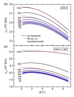
**Figure 10.** Diagonal elements  $\sigma_{xx}$  of the magnetoconductivity tensor of a) a bare CdO layer and b) for a CdO/NiO heterostructure, for various temperatures. Red dashed lines are fits according to Equation (7).
