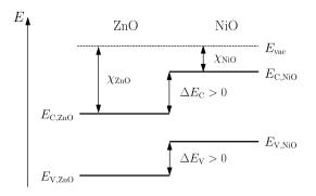
**Figure 2.** Schematic representation of the type-II band alignment between ZnO and NiO.
