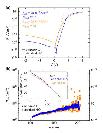
**Figure 3.** a) Current–voltage characteristics for ZnO/NiO heterocontacts from the interface manipulation experiment, and fits in the forward region according to Equation (1). b) Doping profiles for the same contacts, obtained from C-V measurements; the inset shows the corresponding Mott–Schottky plots and extrapolated built-in voltages.
