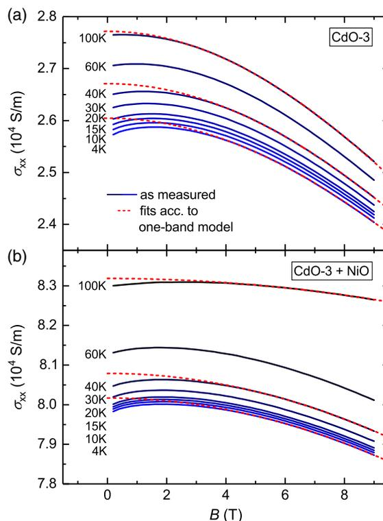
**Figure 10.** Diagonal elements  $\sigma_{xx}$  of the magnetoconductivity tensor of a) a bare CdO layer and b) for a CdO/NiO heterostructure, for various temperatures. Red dashed lines are fits according to Equation (7).
