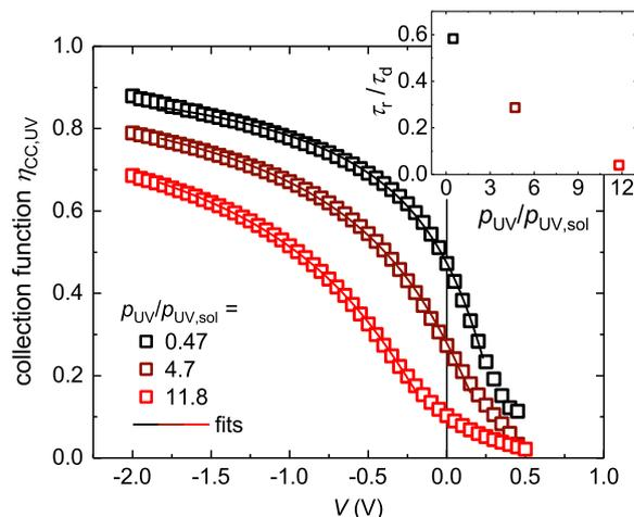
**Figure 5.** Voltage dependence of the carrier collection efficiency of a ZnO/eclipse-NiO solar cell under monochromatic UV excitation for different illumination intensities, and fits according to Equation (6).
