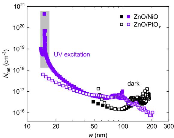
**Figure 6.** Doping profiles of ZnO-based solar cells with an eclipse-NiO and a Schottky front contact, in dark and under illumination with a UV LED ( $p_{opt,UV} = 16 \text{ mW cm}^{-2}$ ), collected at a measurement frequency of 4 kHz.
