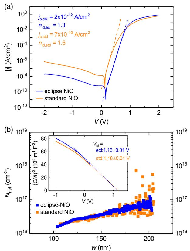
**Figure 3.** a) Current–voltage characteristics for ZnO/NiO heterocontacts from the interface manipulation experiment, and fits in the forward region according to Equation (1). b) Doping profiles for the same contacts, obtained from  $C$ – $V$  measurements; the inset shows the corresponding Mott–Schottky plots and extrapolated built-in voltages.
