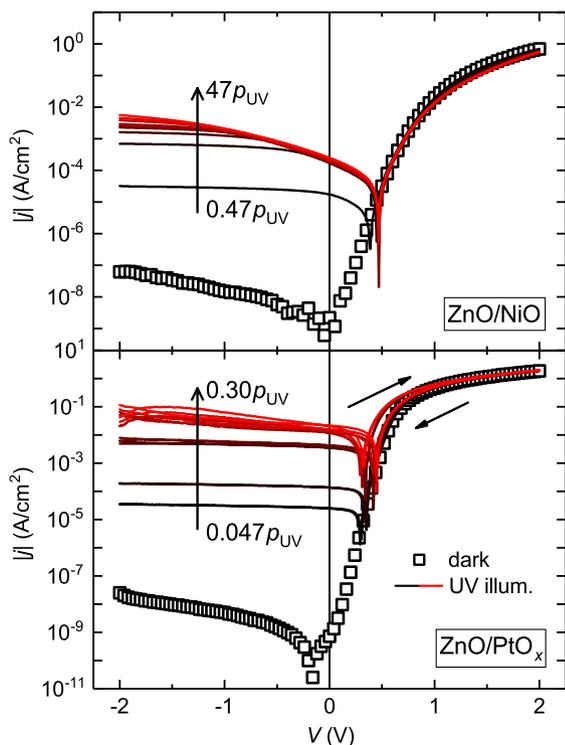
**Figure 4.** Current–density voltage relations of a ZnO/eclipse-NiO (top panel) and ZnO/PtO<sub>x</sub> Schottky (bottom panel) solar cell under UV illumination for different intensities, given relative to the solar terrestrial UV power density. Dark characteristics are also shown.
