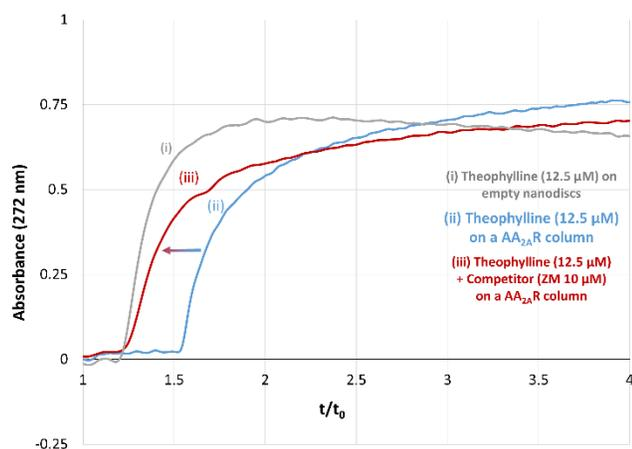
Figure 3. FAC analysis of the competition between theophylline and ZM241385 for the interaction with immobilized AA<sub>2A</sub>R nanodiscs. Frontal affinity breakthrough curves (X-axis in reduced retention time  $t/t_0$ ) of a 12.5 μM theophylline
