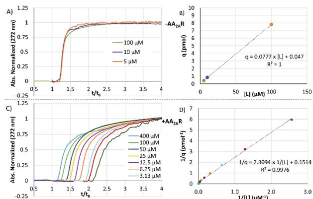
Figure 1. Frontal Affinity Chromatography analysis of the interaction between theophylline and immobilized nanodiscs columns (column dimensions:  $l=8.5 \text{ cm}$  i.d.  $75 \mu\text{m}$ ; applied pressure 12 MPa ( $0.14 \text{ cm}\cdot\text{s}^{-1}$ ))
