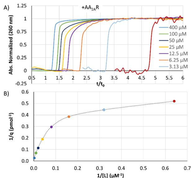
Figure 2. FAC analysis of the interaction between adenosine and immobilized AA<sub>2A</sub>R nanodiscs. (A) Frontal affinity breakthrough curves with adenosine at various concentrations X-axis in reduced retention time  $t/t_0$ ; (B) double reciprocal plot  $1/q$  versus  $1/[L]$  accounting for a two-site model.
