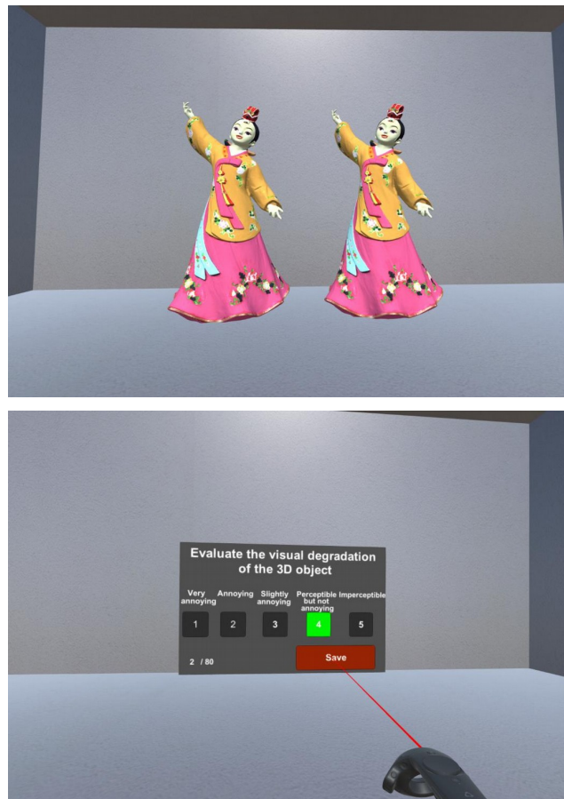
Fig. 3: The experimental environment of our subjective test based on the DSIS method.
