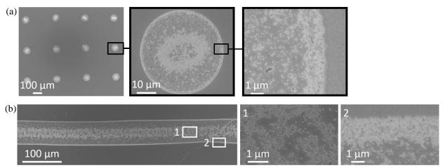
**Figure 3.** (a) Typical SEM images of dry deposits from unfused droplets deposited by inkjet printing, with  $\Delta x > D = 47 \ \mu m$ , at different magnifications. (b) Typical SEM images of dry deposits from fused droplets deposited by inkjet printing, with  $\Delta x = 40 \ \mu m < D$ , at different magnifications.
