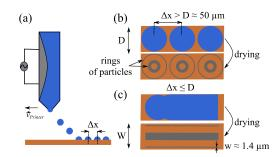
**Figure 1.** Naïve scheme of the inkjet printing process with (a) a cross-sectional view and (b) a top view for drop spacing ( $\Delta x$ ) higher than sessile drop diameter (D). (c) Top view before and after drying for  $\Delta x \leq D$ .
