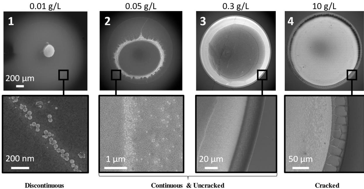
**Figure 2.** Typical SEM-FEG images at different magnifications of the dry patterns formed after the evaporation of sessile drops manually deposited ( $V = 0.5 \mu\text{L}$ ) of SiNP suspensions at different initial concentrations as indicated. The scale bar is the same for all images in the top line. The images in the bottom line are enlargements of the image just above in the area of the external ring.
