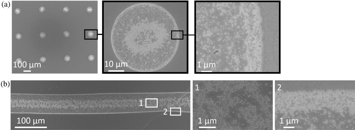
**Figure 3.** (a) Typical SEM images of dry deposits from unfused droplets deposited by inkjet printing, with  $\Delta x > D = 47 \mu m$ , at different magnifications. (b) Typical SEM images of dry deposits from fused droplets deposited by inkjet printing, with  $\Delta x = 40 \mu m < D$ , at different magnifications.
