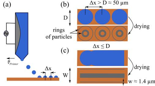
**Figure 1.** Naïve scheme of the inkjet printing process with (a) a cross-sectional view and (b) a top view for drop spacing ( $\Delta x$ ) higher than sessile drop diameter ( $D$ ). (c) Top view before and after drying for  $\Delta x \leq D$ .
