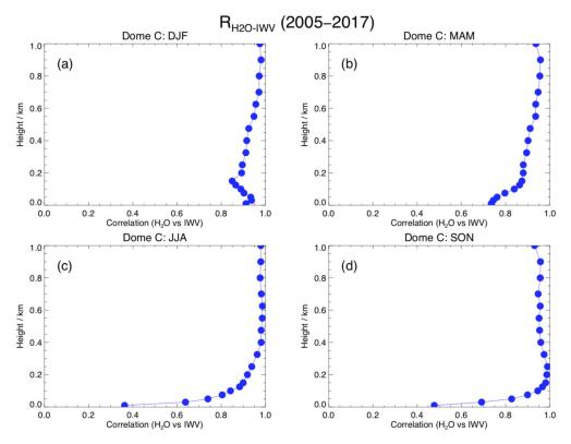
**Figure 4.** Vertical profile of the linear Pearson correlation coefficient  $R_{H2O\text{-}IWV}$  between IWV and water vapor (H<sub>2</sub>O) from radiosondes at Dome C, over the period 2005–2017 in (**a**) DJF; (**b**) MAM; (**c**) JJA; and (**d**) SON.
