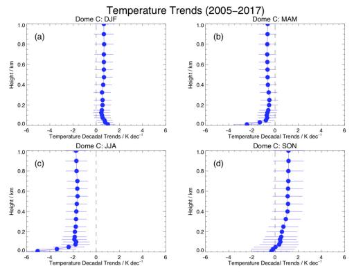
**Figure 8.** Mean profile of the decadal linear trends in temperature at Dome C from radiosondes over the period 2005–2017 in: (a) DJF; (b) MAM; (c) JJA; and (d) SON. Horizontal bars represent 1- $\sigma$  error.
