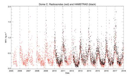
**Figure 1.** Time evolution of daily-averaged IWV (kg m $^{-2}$ ) measured at Dome C from 2005 to 2017 by the radiosondes (red filled circles) and from 2009 to 2017 by H<sub>2</sub>O Antarctica Microwave Stratospheric and Tropospheric Radiometers (HAMSTRAD) (black stars).
