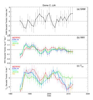
**Figure 11.** Multidecadal variability of the 10-year trends of (a) the SAM index, (b) the IWV and (c) the near-surface temperature ( $T_{2m}$ ) from the MERRA2 (red), ERA interim (dark blue), ERA5 (light blue) and JRA-55 (green) reanalyses above Dome C from 1980 to 2017 in winter (JJA). Superimposed are the 10-year trends of the IWV (b) and the 10-m temperature (c) from the radiosonde data set (orange) from 2005 to 2017. Vertical bars represent 1- $\sigma$  error.
