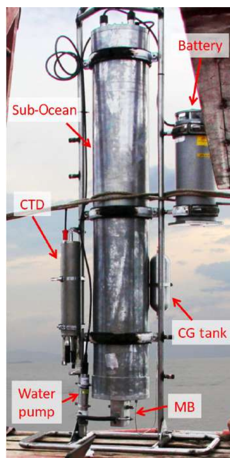
Figure 2. A picture of the Sub-Ocean instrument and the full assembly. The sensor is mounted on a metal frame. The main tube at the center is 150 cm long and 28 cm in diameter. The membrane block (MB) at its bottom is connected to the water pump to ensure a constant flow of water against the membrane. The carrier gas (CG) tank is attached to the metal frame and connected with a 1/8 in. stainless-steel tube at the instrument. An STR battery pack and a CTD sensor were also attached to the metal structure. The total weight of the assembly is 120 kg with about -50 \text{ kg} of buoyancy.
