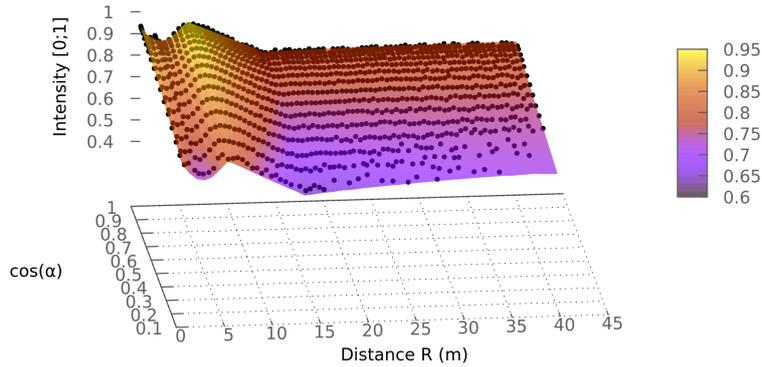
Figure 6: Colored surface regression with raw intensity (black points) as a function of distance and cosine of incidence angle.
