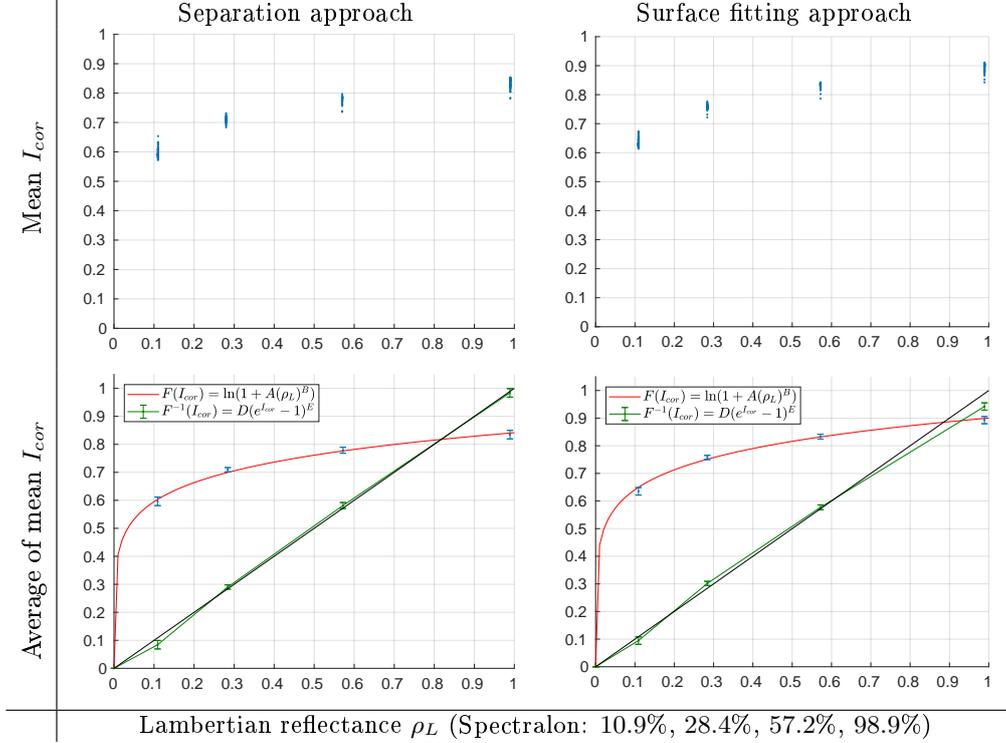
Figure 10: Top) Mean corrected intensities of the four Spectralon parts for various ranges and incident angles. Bottom) Average of mean corrected intensities for each Spectralon part (blue), logarithmic approximation (red curve), and linearized  $I_{cor}$  values compared with perfect linear line (black)
