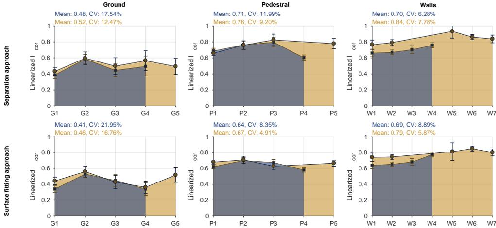
Figure 11: Separation and fitting approaches applied on the two previous heterogeneous 3D clouds. Comparison of linearized corrected intensities for various surfaces, on a  $[0;1]$  scale.
