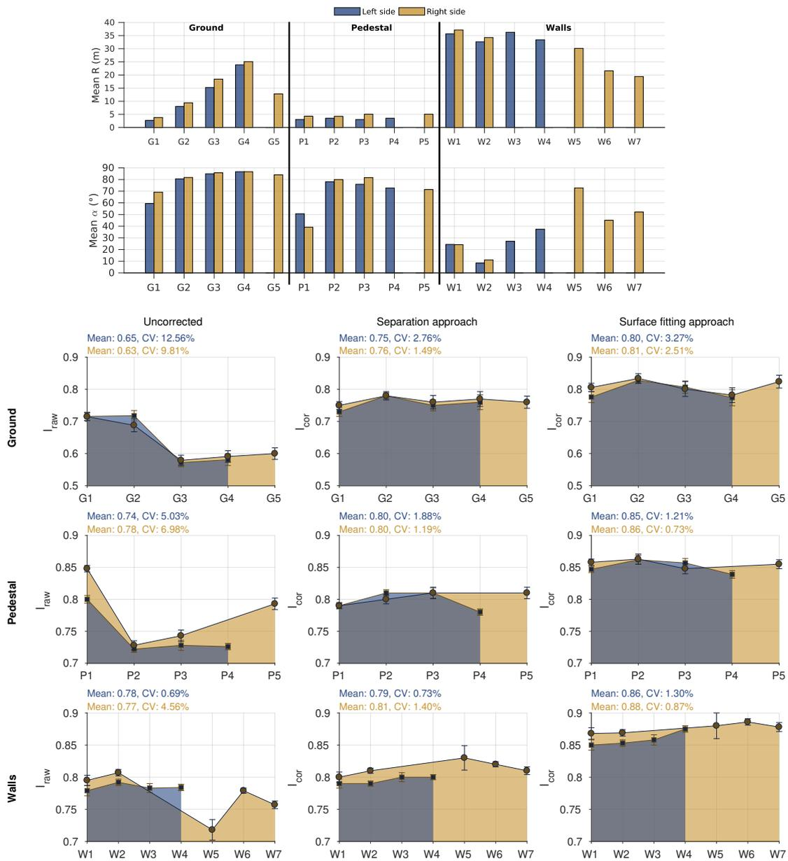
Figure 9: Separation and sphere fitting intensity correction approaches applied on two scans of a heterogeneous point cloud. Top) Selected area mean distances and incidence angles. Bottom) Comparison of area mean intensities before and after correction.
