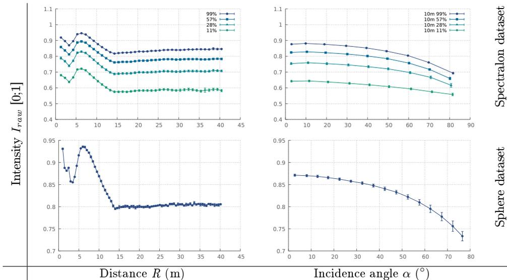
Figure 4: Raw intensities measured of the Spectralon and sphere targets as a function of distance and incidence angle. Left) Mean raw intensities as a function of distance for the four Spectralon parts and sphere target, with a maximal incidence angle of  $15^\circ$ . Right) Mean raw intensities as a function of incidence angle for the four Spectralon parts at 10 m by classes of  $10^\circ$ , and for the sphere target at 10 m by classes of  $5^\circ$ .
