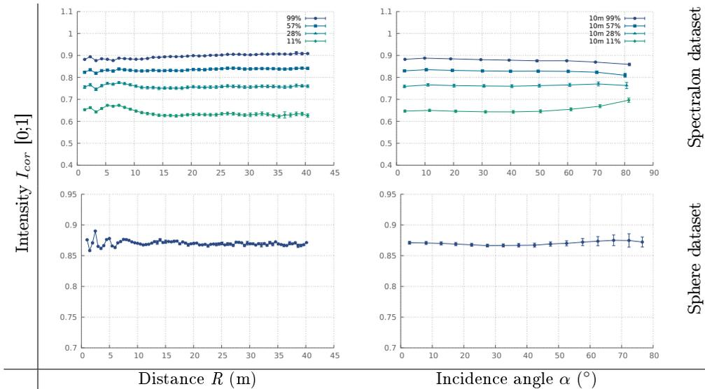
Figure 7: Surface fitting approach applied on the Spectralon and sphere calibration datasets as a function of distance and incidence angle. Left) Mean corrected intensities as a function of distance for the four Spectralon parts and sphere target, with a maximal incidence angle of  $15^\circ$ . Right) Mean corrected intensities as a function of incidence angle for the four Spectralon parts at 10 m by classes of  $10^\circ$ , and for the sphere target at 10 m by classes of  $5^\circ$ .
