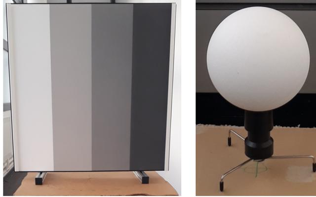
Figure 3: Photography of the used targets: Spectralon with 99%, 57%, 28% and 11% reflectivity surfaces, and sphere.
