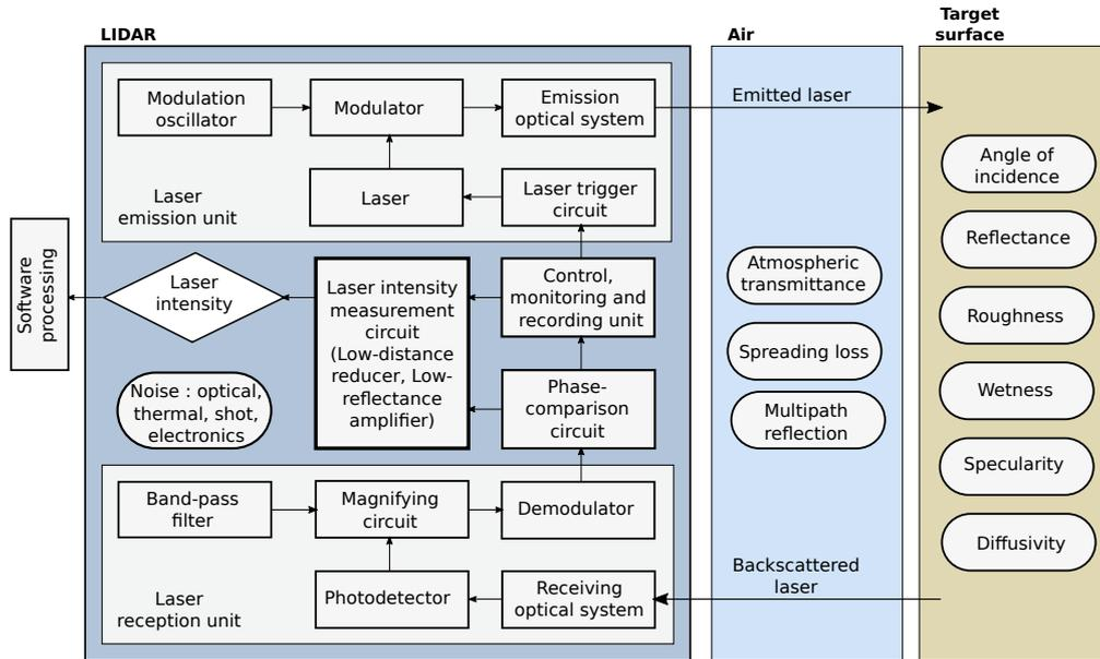
Figure 2: LiDAR FMCW intensity measurement processes with phenomena affecting the backscattered signal. Squares represent the signal processing steps and rounded squares the different sources of signal modifier.
