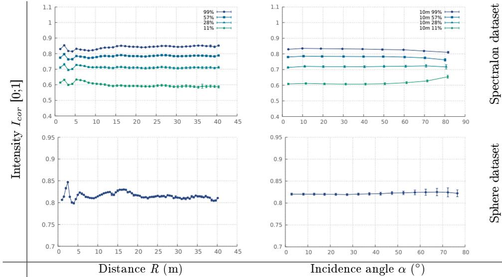
Figure 5: Separation approach applied on the Spectralon and sphere calibration datasets as a function of distance and incidence angle. Left) Mean corrected intensities as a function of distance for the four Spectralon parts and sphere target, with a maximal incidence angle of  $15^\circ$ . Right) Mean corrected intensities as a function of incidence angle for the four Spectralon parts at 10 m by classes of  $5^\circ$ , and for the sphere target at 10 m by classes of  $5^\circ$ .
