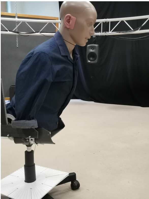
Figure 10. Installation for the 20^\circ recording at the SCRIME. Although the manikin is surrounded by loudspeakers, only the one in front of it is used for the measurements.
