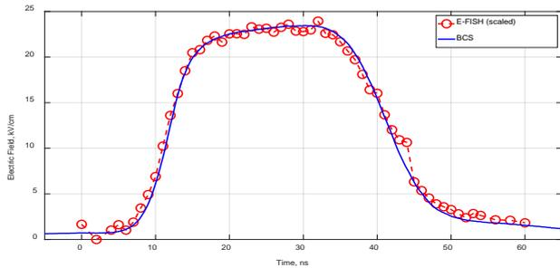
Fig. 3. Time evolution of (square rooted) E-FISH signals (produced by 2.8 ns pulses) appropriately scaled and plotted together with the field evolution measured by the back current shunt (BCS). The time-varying field is imposed by applying 30 ns (FWHM) HV pulses with a rise time of about 8 ns.
