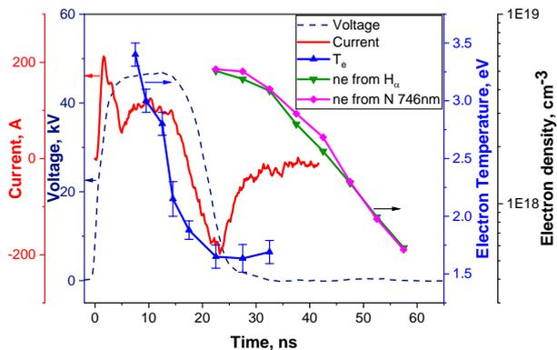
Fig. 4. Synchronized electron density and temperature measurements. Nanosecond SDBD Discharge in 7 bar  $N_2$  at positive polarity of the high-voltage pulse,  $U = 47$  kV.
