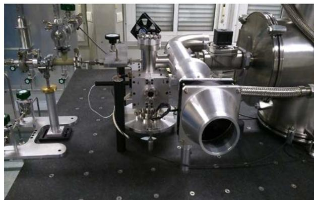
Fig. 2. Discharge cell for high pressure ( $P < 15$  bar) high temperature ( $T < 700$  K) nanosecond SDBD
