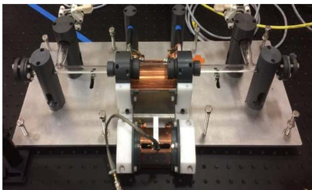
Fig. 1. Discharge tube for laser diagnostics in 20-100 mbar fast ionization waves
