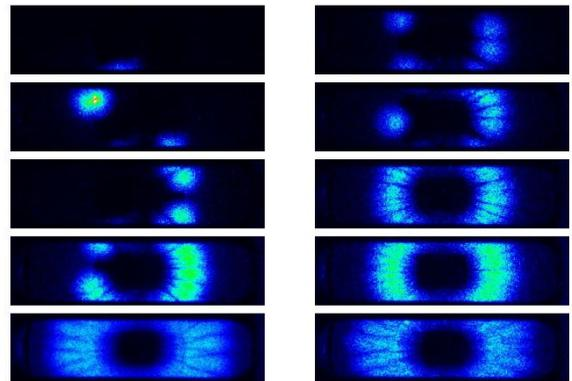
Fig. 5. Combustion waves initiated in 5 bar (left) and 3 bar (right)  $H_2$ :air ( $ER=0.6$ ) near the surface of the dielectric. The high voltage electrode is a disk 20 mm in diameter.
