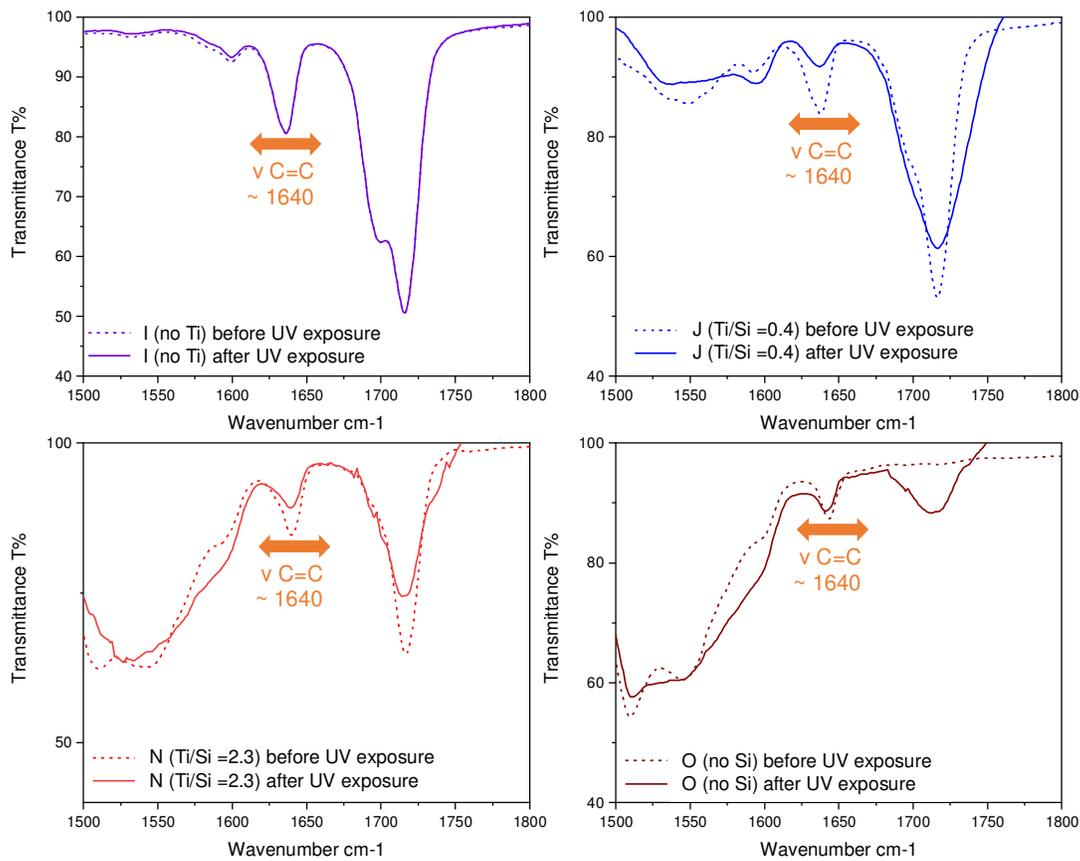
**Fig. 6** IR spectra on films with different molar ratios Ti/Si (resins I, J, N, O) before and after UV exposure, focusing on the C=C elongation band at 1640 cm<sup>-1</sup>
