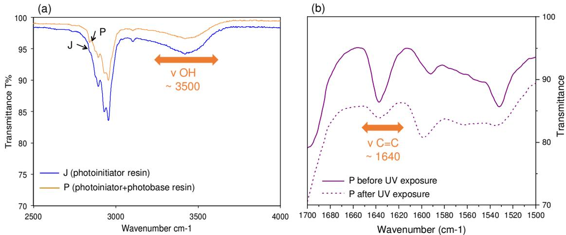
**Fig. 7** (a) IR spectra on films of the photobase resin (resin P) and the photoinitiator resin (resin J) as reference, focusing on the OH elongation band at  $3500\text{ cm}^{-1}$  (b) IR spectra on films of the photobase resin (resin P) before and after UV exposure, focusing on the C=C elongation band at  $1640\text{ cm}^{-1}$
