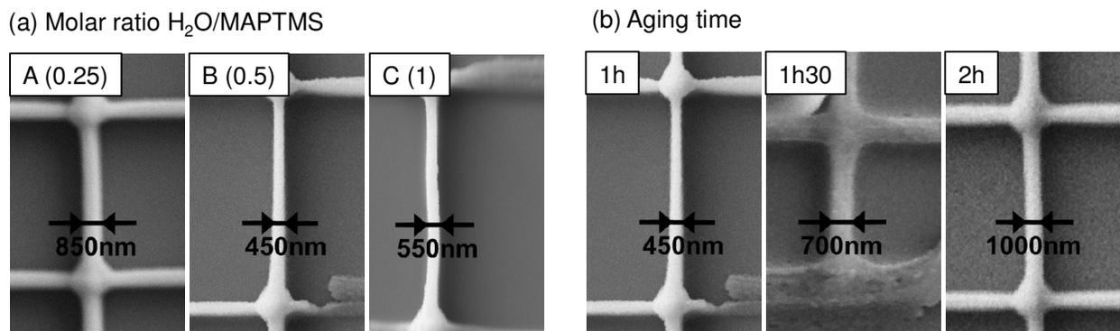
**Fig. 4** Microlines printed at  $70\mu\text{W}$ , obtained from resins in function of different experimental preparation conditions (a) Variation of molar ratio  $\text{H}_2\text{O}/\text{MAPTMS}$ , after an aging time of 1h (resins A, B and C) (b) Variation of aging time (resin B)
