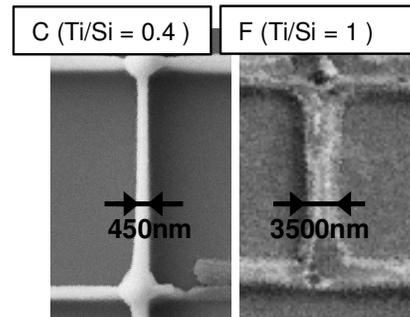
**Fig. 3** (a) Example of microgrids obtained from resins at different molar ratios Ti/Si with TiP and TiB (resins C, F, J, L, N) (b) Comparison between microlines obtained from resins with TiP and TiB, printed at 70 μW, after an aging time of 1h (resins F, L) (c) Microlines obtained at 70 μW from resins at different molar ratios Ti/Si with TiP, after an aging time of 1h (resins C, F)
