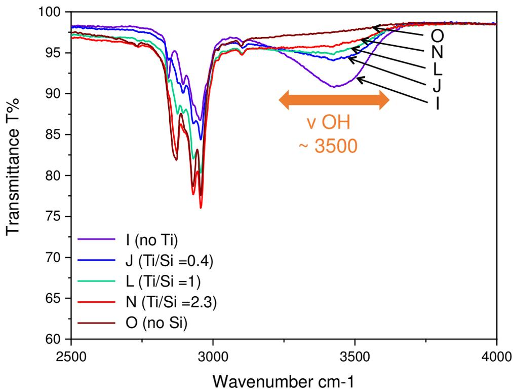
**Fig. 5** IR spectra of films for different molar ratios Ti/Si (resins I, J, L, N, O), focusing on the OH elongation band at  $3500\text{ cm}^{-1}$
