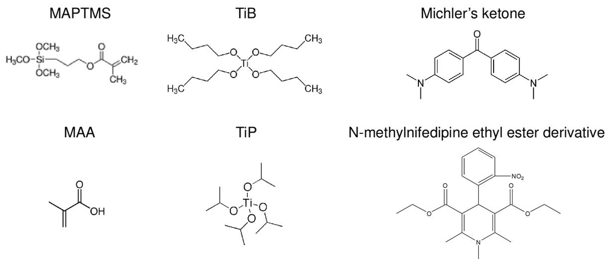
**Fig. 1** Reactants used in the different hybrid resins
