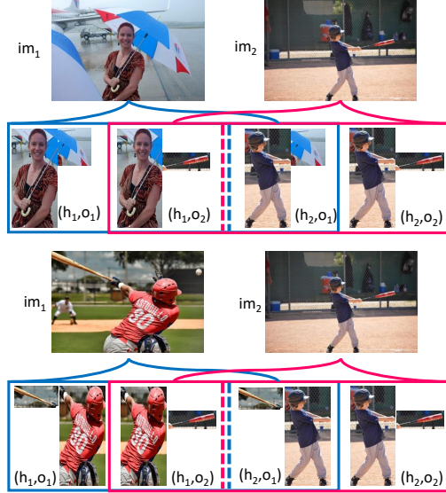
Figure 3: Illustration of HOI element swapping. Top: Object classes from the two images are different. Bottom: same object class in the two images. Swapped pairs (h_i, o_j) are negatives due to wrong object class (top) or wrong spatial layout (bottom).
