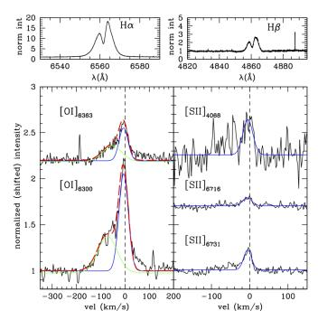
**Fig. 5.** FEROS spectrum of RCrA. *Top panels*: regions around Hα and Hβ lines. *Bottom panels*: regions around [O I] $\lambda$ 6716/6731 and [S II] $\lambda$ 4068/6716/6731 forbidden lines. The colored Gaussian profiles in the *bottom panels* refer to the multiple component deconvolution: in green, the HVC, in blue, the LVC, in red, the sum of the two components.
