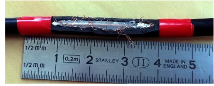
Fig. 8. Chafing soft fault (chafing of the shield and the insulator) created on the RG-58 coaxial cable.
