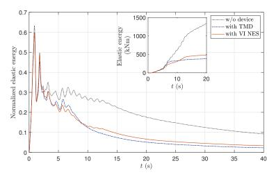
Figure 8: Cumulative elastic energy for the uncontrolled structure, for the structure controlled by the VI NES, and for the structure controlled by the TMD. Normalization is performed with respect to the injected energy.
