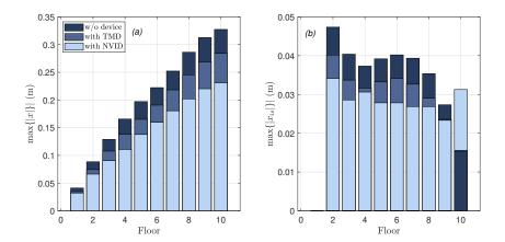
Figure 9: Seismic response at each floor of the frame structure controlled by the VI NES and the TMD. (a) maximum displacement,  $\max\{|x_i\}|$ , and (b) maximum inter-story drift,  $\max\{|x_{is}\}|$ .
