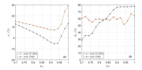
Figure 10: Sensitivity analysis on the variation of the stiffness of the primary structure. (a) Reduction of the maximum 10-th floor lateral displacement relative to the ground. (b) Reduction of the cumulative elastic energy.
