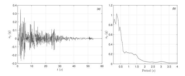
Figure 4: El Centro NS (1940) earthquake: (a) time history and (b) elastic response spectrum (damping ratio 2 %).
