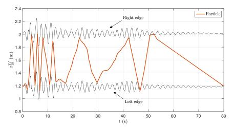
Figure 7: Time history of the displacement of the opposite walls and of the particle of VI NES.
