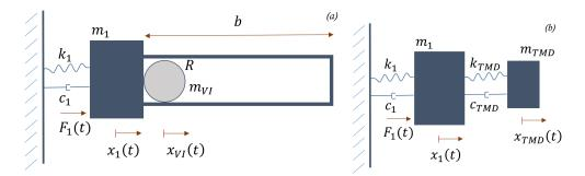
Figure 1: Schematic representation of (a) a VI NES and (b) a TMD.
