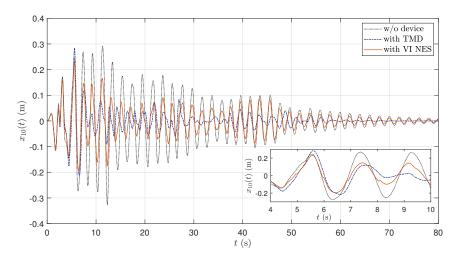
Figure 6: Time history of the lateral displacement of the 10-th floor. Comparison between the uncontrolled structure (w/o device) and the structure controlled by the VI NES and the TMD.
