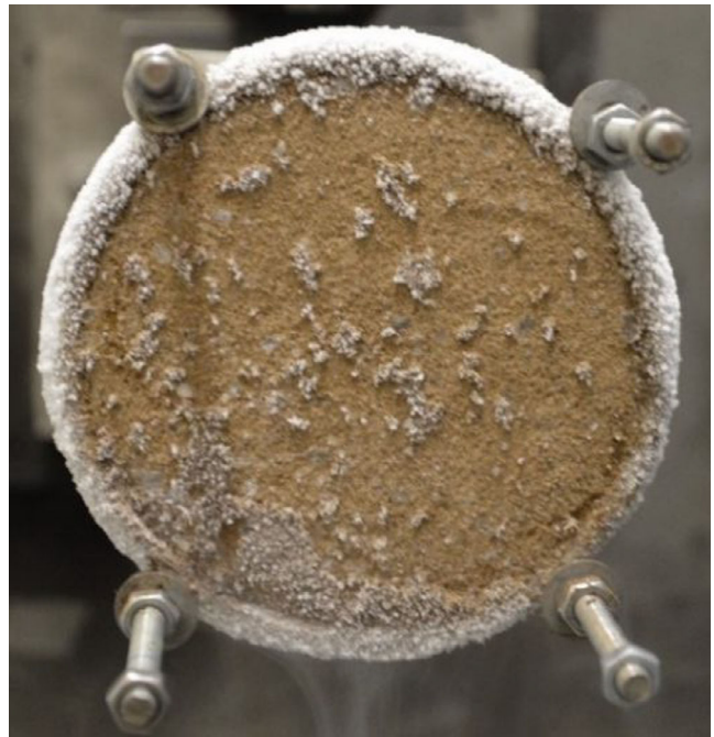
Fig. 1. A 100 mm diameter, stainless steel can containing a frozen ~50:50 mixture of finely crushed CO 2 ice and JSC-1 Martian regolith simulant.
