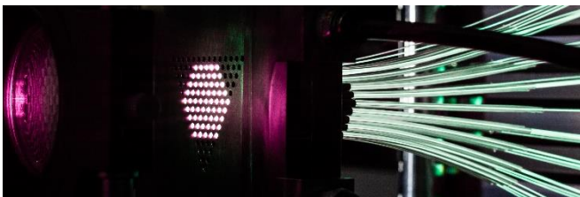
Fig. 1. XCAN laser head (center), collimating microlens array (left) and 61 Yb doped fiber bundle (right). More details about the experimental setup of the CBC of 61 fiber amplifiers are given in reference [10].
