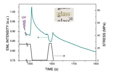
**Figure 2.** Uniaxial compression test, with the preliminary UV irradiation being performed under load. A  $4 \times 4 \times 4.47$  mm<sup>3</sup> parallelepiped sample was UV-irradiated for 30 s under a 26 MPa compression load. The sample was loaded for 1500 s, unloaded at 1500 s and further reloaded at 1575 s for 10 s. The inset shows the bar from which were cut the specimens for mechanical testing.
