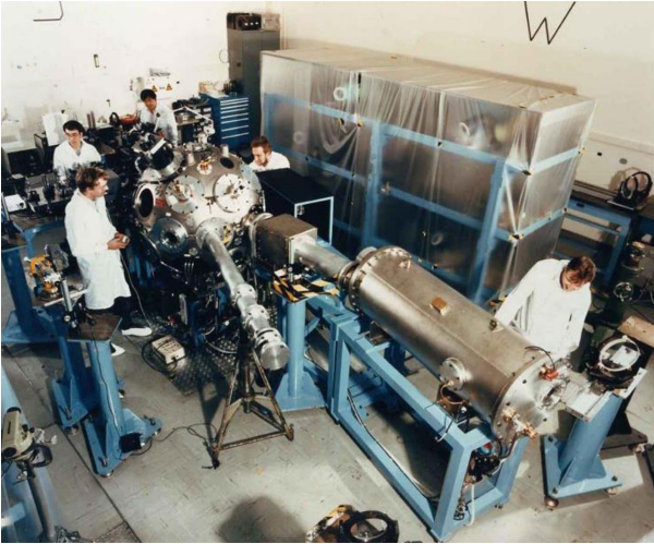
Figure 3. The Vulcan 100 TW laser from the early/mid-1990s showing the first ever single-pass CPA compressor system with one grating in air (centre) and the second in vacuum (bottom right) (picture courtesy of STFC Rutherford Appleton Laboratory).
