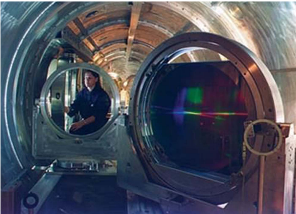
Figure 4. Inside the Nova Petawatt compressor chamber (picture courtesy of LLNL).
