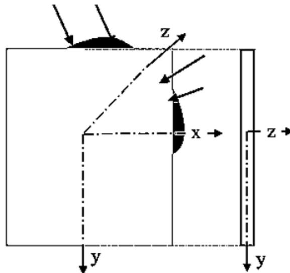
Fig. 1. Solid in a plane stress.
