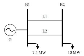
Figure 3: Test system with 4 components (system order  $n = 2^4 = 16$ ).
