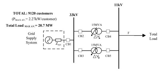
Figure 8: Generic MV substation model – 10PCs.
