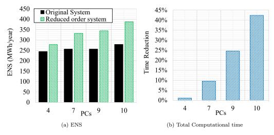
Figure 9: Trends of reliability accuracy and computational time of the MOR methodology with respect to the original size, for the generic MV substation presented in Fig. 8.
