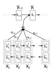
Figure 2: Schematic of the alignment model adapted from Bahdanau *et al.* (2014)
