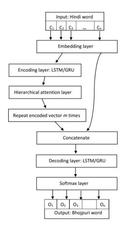
the encoder-decoder network incorporating the alignment-based attention decoder.
