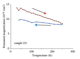
**Fig. 3.** Thermal demagnetization in the absence of magnetic field for the sample D1 from 30 to 250 K (upper curve). The initial saturation remanent magnetization was acquired at 10 K in a magnetic field of 1 T. The demagnetization is followed by cooling between 250 and 30 K in the absence of a magnetic field (lower curve).
