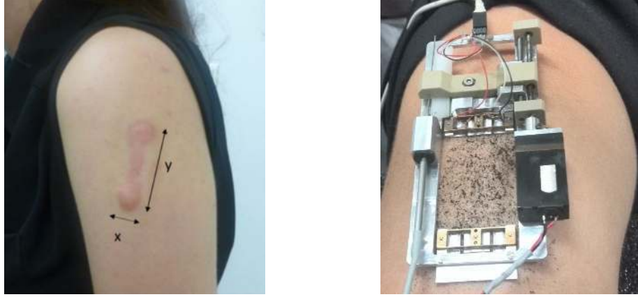
(a) Keloid scar located on the left-upper arm ( X = 15 \text{ mm} , Y = 47 \text{ mm} ). (b) Extensometer. The speckle pattern is used for capturing the displacements.
