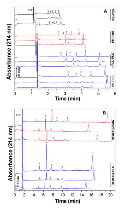
Figure 2. Inter-capillary reproducibility of 5-layers SMIL coatings (PB-PLC,  $\varepsilon$ -PLL-PLC, PB-PMA, PB-PSS couples (A) or DEAEDq-PLC, DEAEDq-PMA couples (B)) for the electrophoretic separation of 5 test proteins in 0.5 M acetic acid. 3 different capillaries were tested for each coating (*n*=7 for each capillary). Only the first separation on each capillary in shown. Experimental conditions as in Figure 1.
