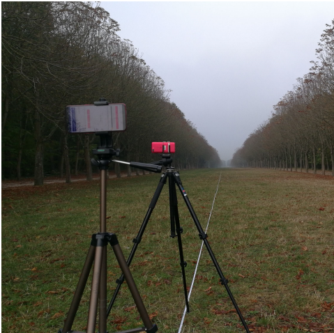
Figure 4: Photography of the experimental procedure. Both smartphones run the Ocat application, and we move one of the tripods according to a chosen stepping along the measuring tape (white line on the ground).
