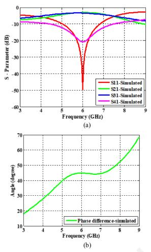
Fig. 4: S- Parameter result of the coupler (simulated), (a) the magnitude (dB); (b) the Phases difference (degrees).
