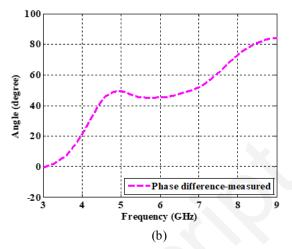
Fig. 5: The S- Parameter for the Proposed Coupler (measured), (a) Magnitude (dB); (b) Phases difference (degrees).
