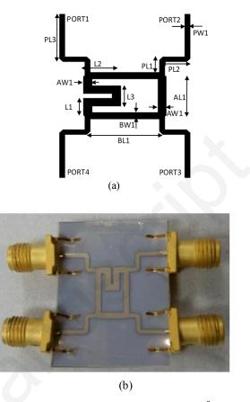
Fig. 3: (a) Schematic layout of the proposed  $45^{\circ}$  coupler, (b) photograph of the front view of the fabricated coupler
