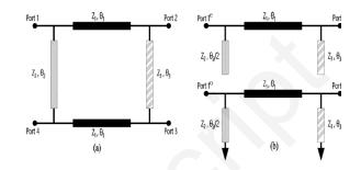
Fig. 2: (a) Schematic diagram of the proposed coupler; (b) The even/odd mode equivalent.
