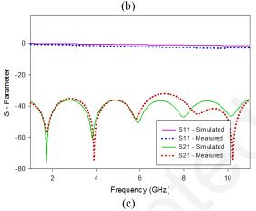
Fig. 1. (a) The Brother printer DCP–J140w (b) layout and photograph of a 50 $\Omega$  microstrip TL simulated and prototyped with the PET substrate. (b): The S- parameter for the microstrip TL.
